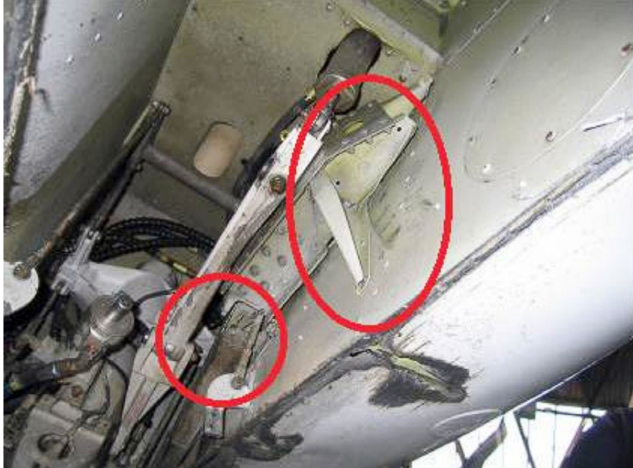
Figure 3. Forward gear wheel well showing the fracture area and the loss of the rivets that hold the drag link in place
