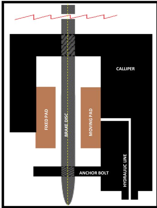
This is the position of the brake at rest.
