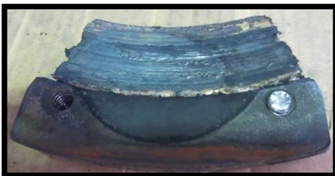
*Figure 13: Fixed pad after the accident.*
