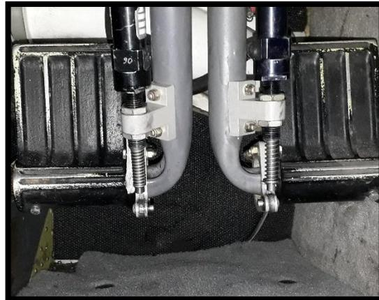
*Figure 16: Master actuator pistons of the co-pilot's brake pedal.*
