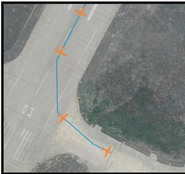
According to the GPS trace, the aircraft taxied back along the runway for 1 minute and 40 seconds, covering approximately 1,150 metres, until it reached the holding point for taxiway C5, as can be seen in the figure. Based on the above, the average speed during the taxi was approximately 40 km/h.
