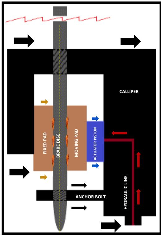
As the moving pad cannot continue forward after making contact with the brake disc, the entire calliper moves sideways, sliding the anchor bolts through the holes in the landing gear leg plate (torque plate bushings). It then uses the moving pad, which is already pressing on the brake disc, as a support point to drag the fixed pad forward until it makes contact with the other side of the disc, braking the aircraft.
