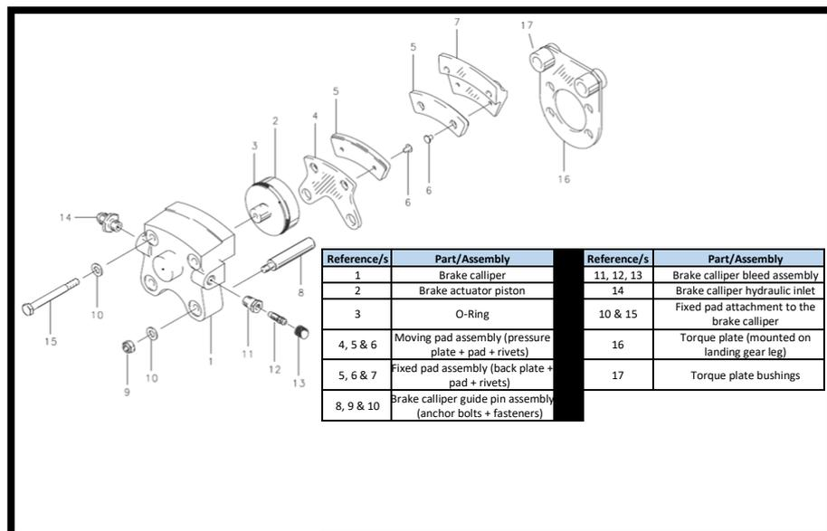
Figure 3: Diagram of the aircraft's brake.
