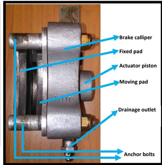
Figure 20: Brake (plan view).
