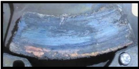
*Figure 12: Moving pad after the accident.*
