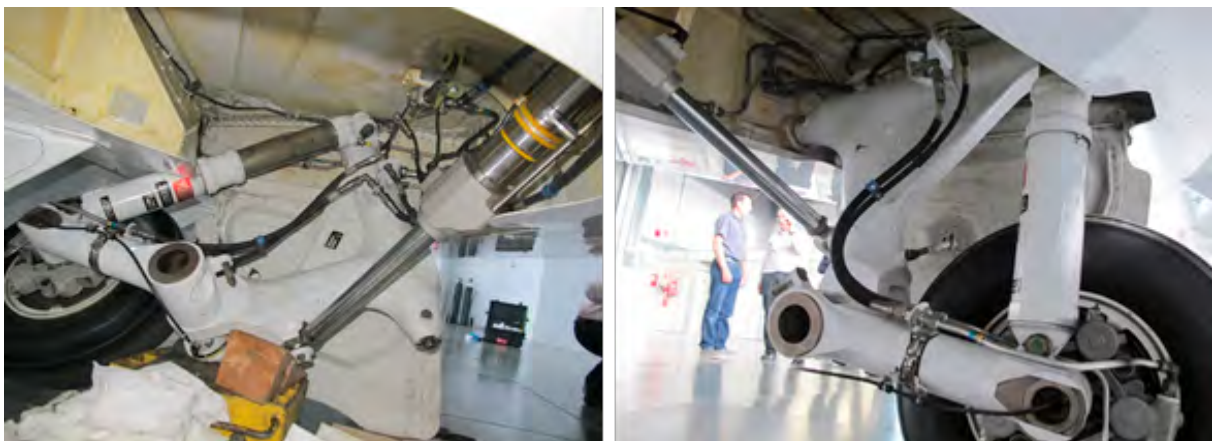
Figure 2 – Left leg outside the wheel well (l), and right leg in its normal extended position (r)
