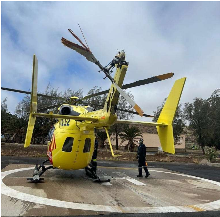
Fig no. 1. - Condition of the helicopter's tail rotor and vertical stabiliser.
