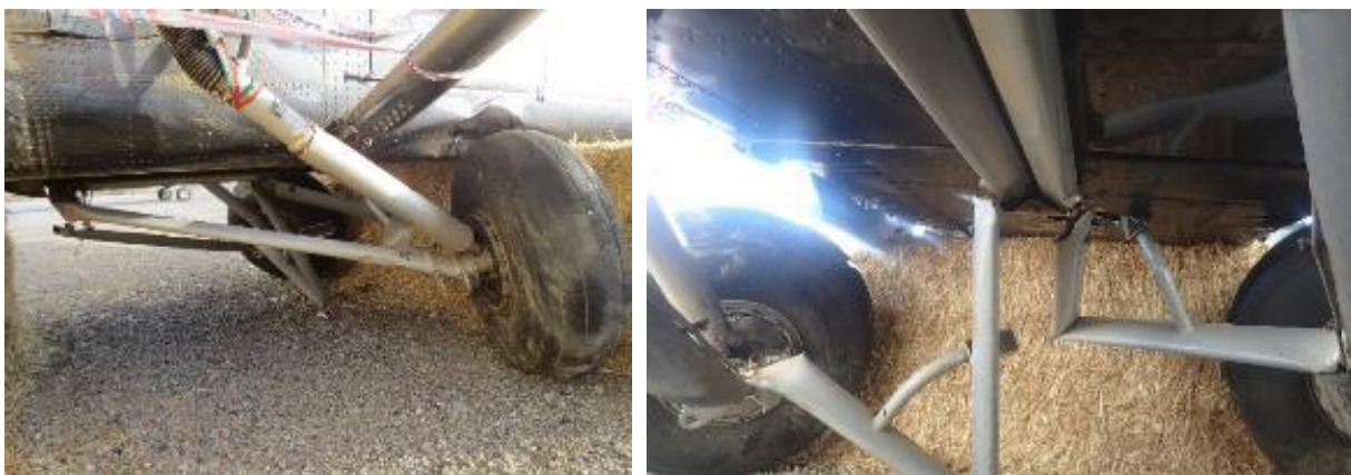
Photograph 4. Damage to landing gear
