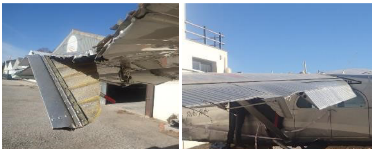
Photograph 3. Damage to flap and aileron on left wing
