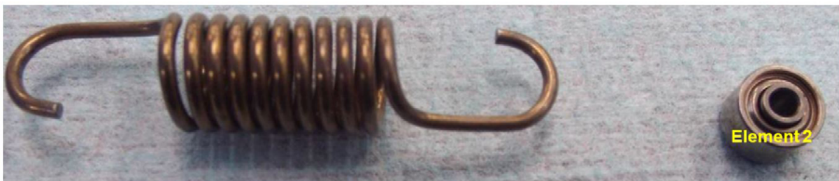
Photograph 9. FCU components: element 1 – governor spring, and element 2 – enrichment lever bearing
