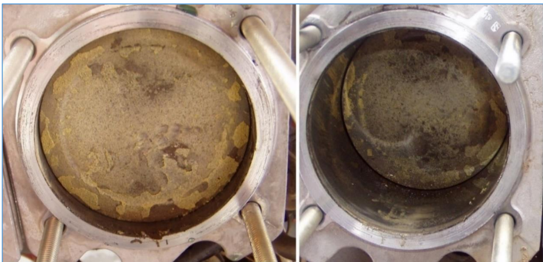
Figure 7. Residue in cylinders 1 & 2
