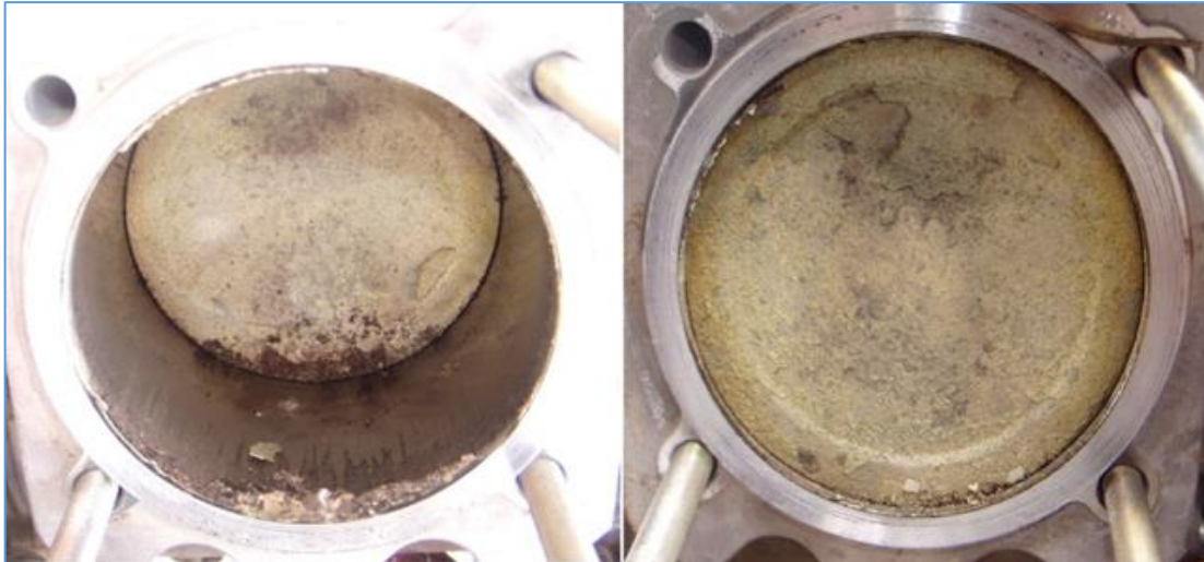
Figure 8. Residue in cylinders 3 & 4
