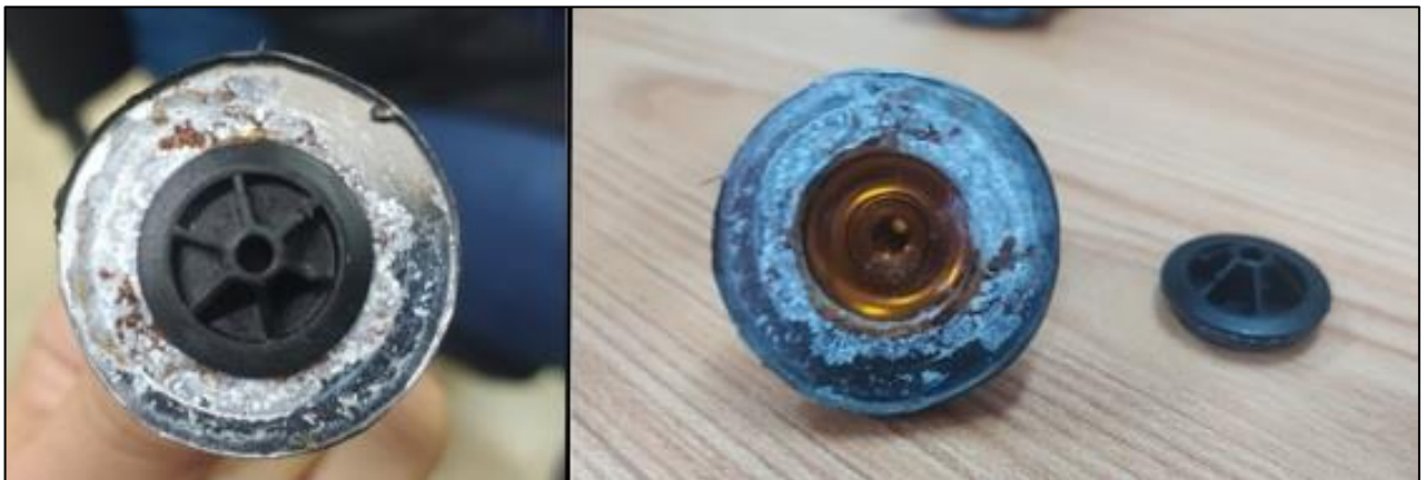
Figure 10. Interior of the low fuel pressure warning sensor
