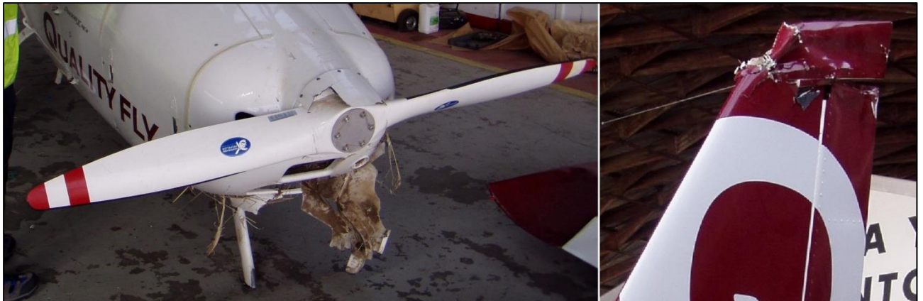
Figure 1. Damage to the landing gear and vertical stabiliser
