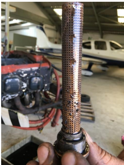
Photograph 19: Oil filter with metallic particles
