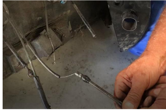
Photograph 13. Mixture controller cable in the rich mix position
