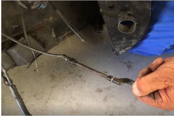
Photograph 12. Mixture controller cable in the lean mix position
