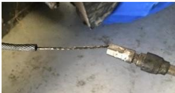
Photograph 14. Detail of the non-crimped mixture controller cable
