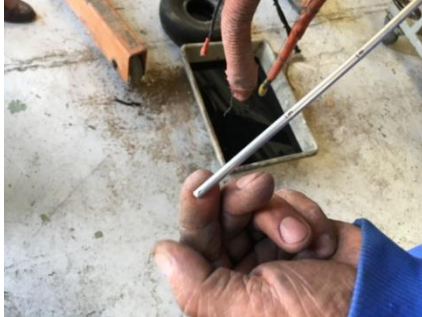
Photograph 17: Oil dipstick and remaining oil in the float bowl
