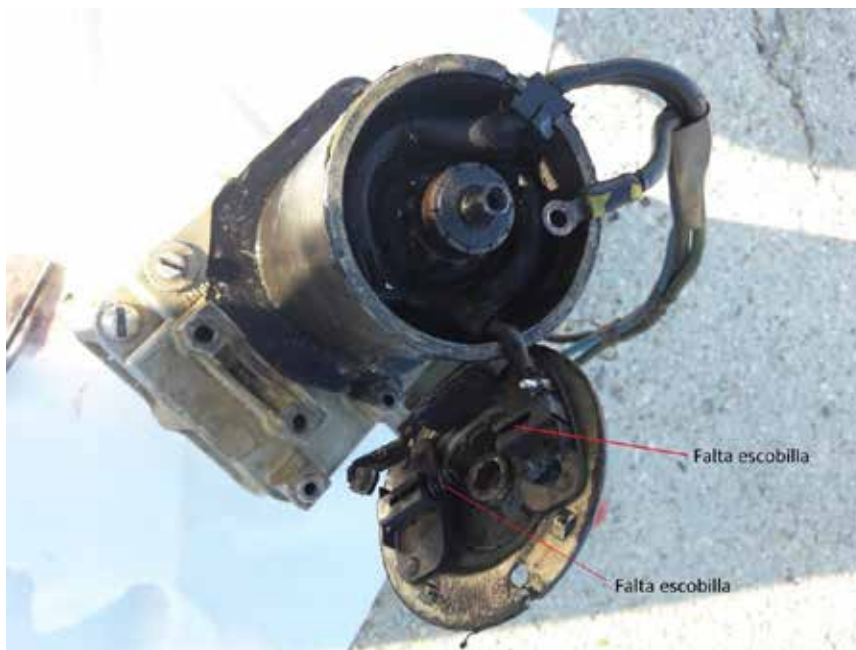
Fig. 6.- Condition of the electric pump
