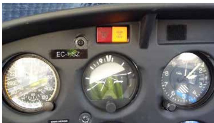
Fig. 2.- Amber gear-transit light and red gear warning light
