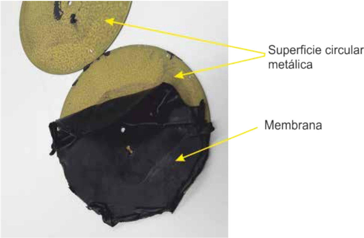
Fig. 12.- Internal view of diaphragm assembly
