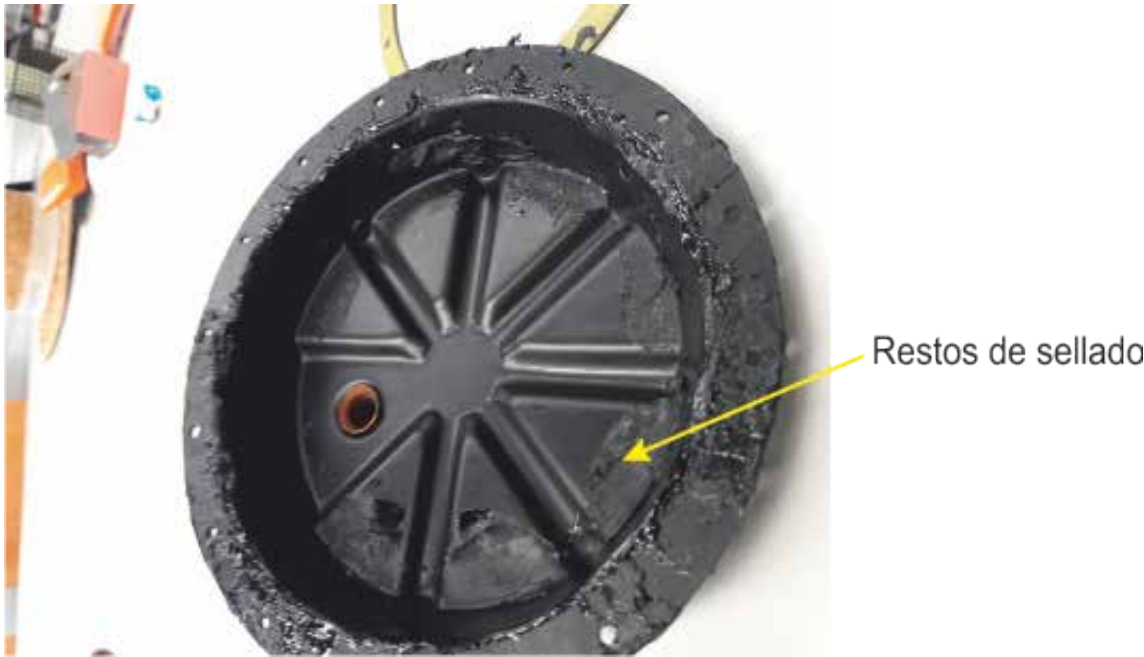
Fig. 11.- Half of casing to which diaphragm assembly had adhered
