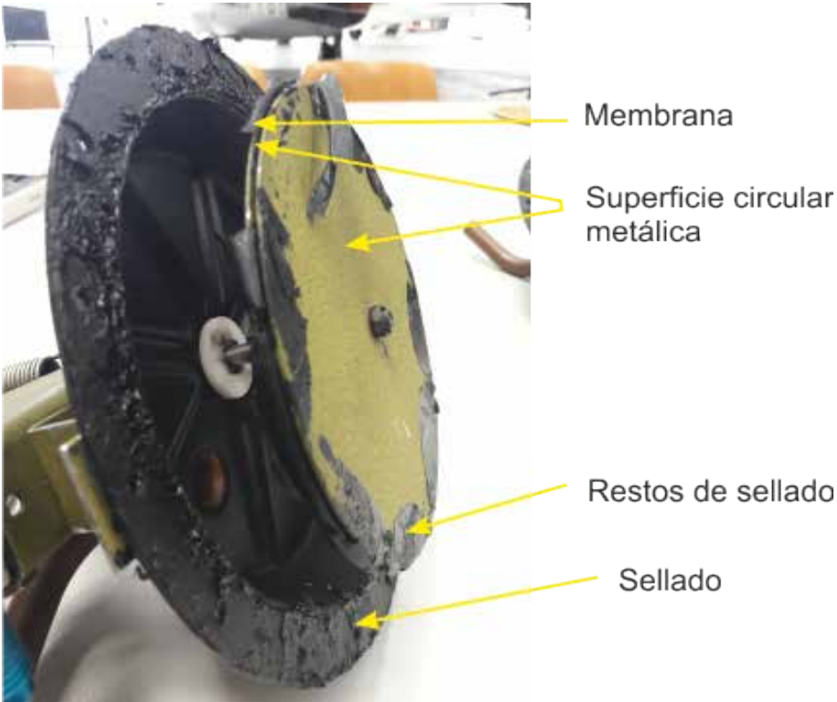
Fig. 10.- Diaphragm assembly detached from the casing
