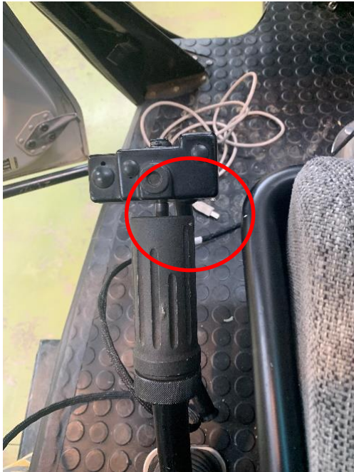
Photograph 24: Twist grip installed for training in the left-hand position occupied by the instructor. Absence of yellow mark highlighted with a red circle.
