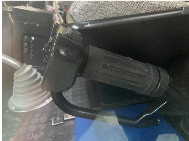
Photograph 24: Twist grip installed for training in the left-hand position occupied by the instructor. Absence of yellow mark highlighted with a red circle.
