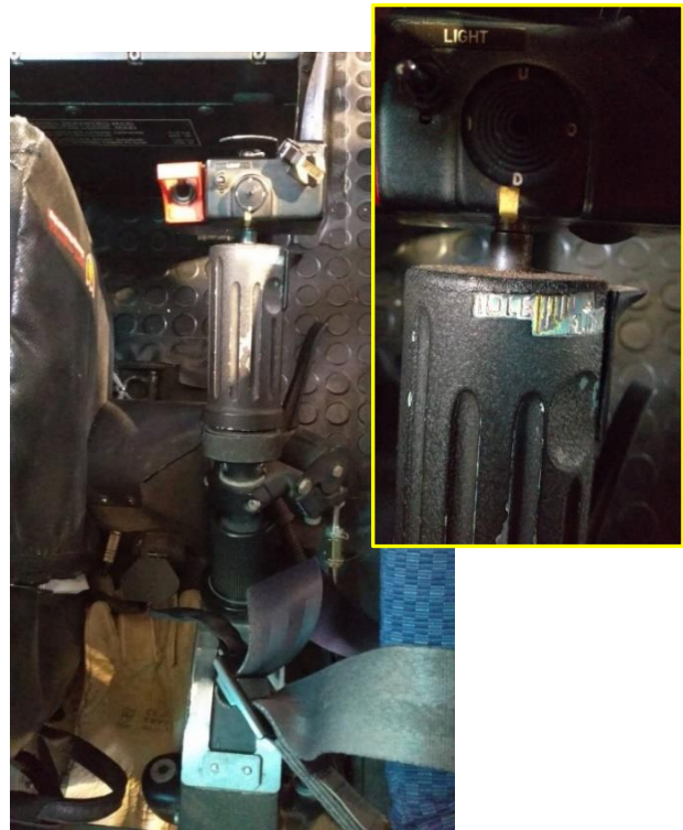
Photograph 9. Collective in the 2B1 model and close-up of the twist grip
