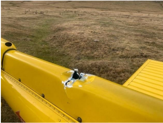
Photograph 16. Tail rotor drive shaft fairing
