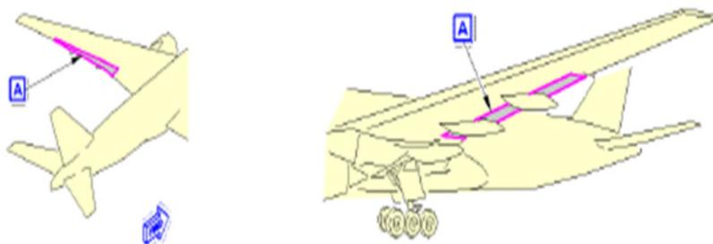
Image 1: Location of the outboard flap on the left wing
