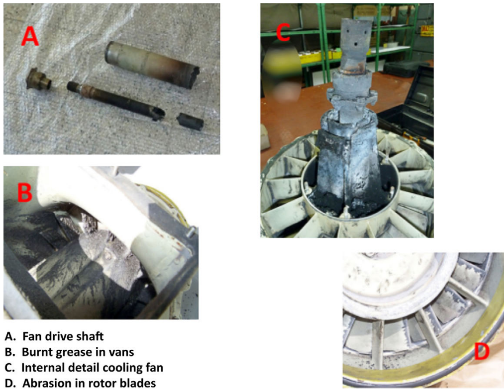
Figure 3. Close-up of the fan components
