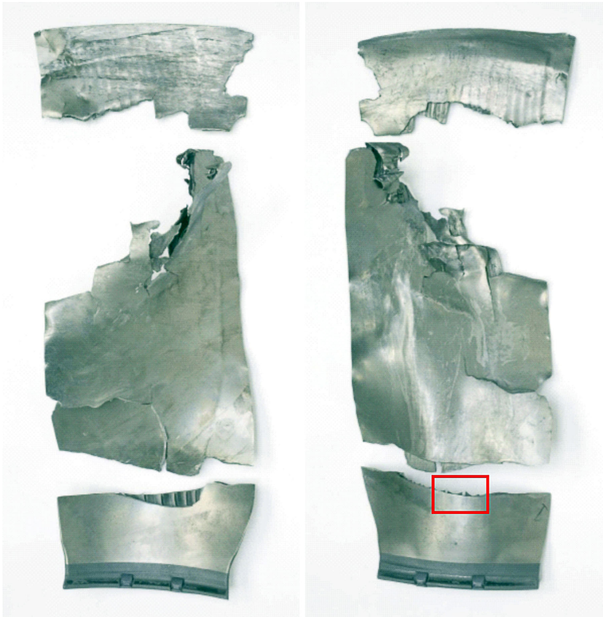
Figure 6. Reconstructed blade (left – pressure concave panel, right – suction convex panel)
