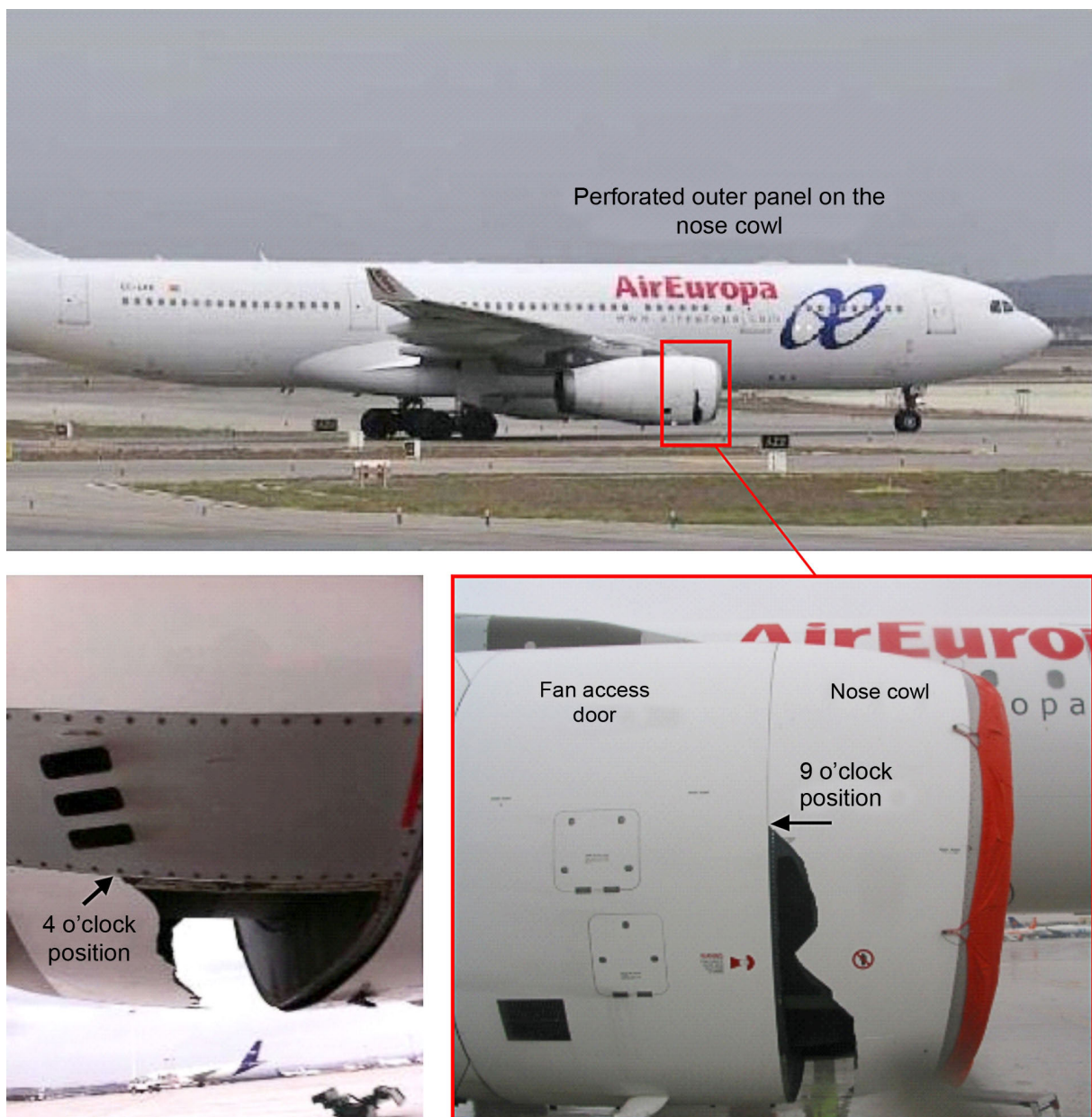
Figure 1. Aircraft after the incident (view from the side of engine n.º 2)
